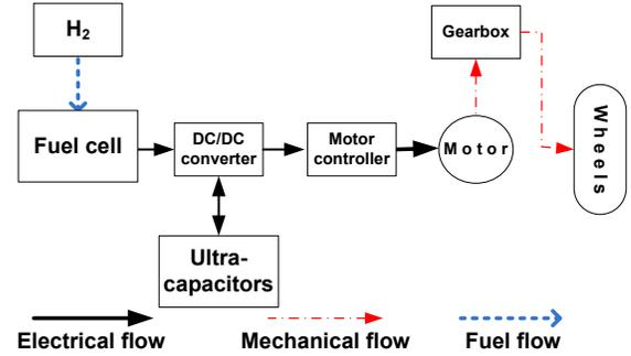
Figure 1: Main components and flows of vehicle's powertrain
