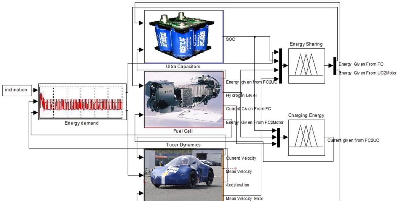
Figure 2: Simulink model of the suggested fuel management system
