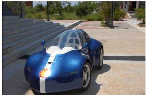
Figure 1: TUCer fuel cell prototype vehicle, version ER11
