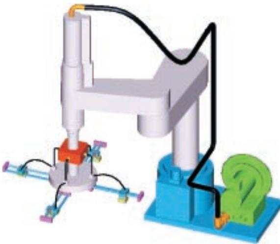
Fig. 3 The reconfigurable gripper prototype mounted on an Adept robot arm
