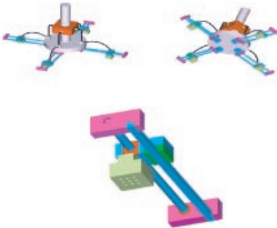
Fig. 2 Design of the reconfigurable gripper system
