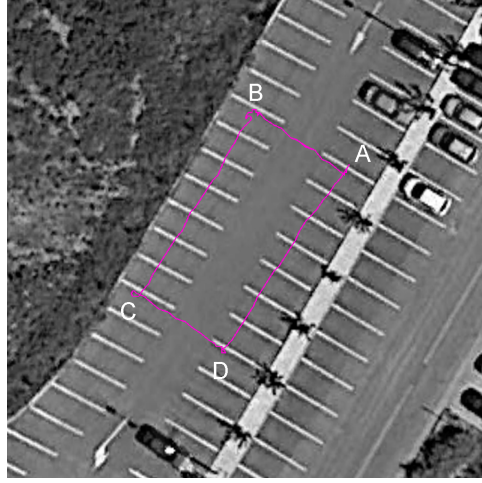
Fig. 5. The experimental testing scenario for the Waypoint Movement node was to move through the multiple POIs, A, B, C, D. The actual path followed by the robot is shown in pink. The experiment was conducted using half speed - approximately 5.2km/h. The path followed by the robot is shown in magenta. The mean error value, i.e. the distance from the straight path lines, was 0.8m and it is due to errors at the GPS readings.
