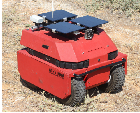
Fig. 1. The reDevil robot: an upgraded ATRV-mini outdoors robotic vehicle.
