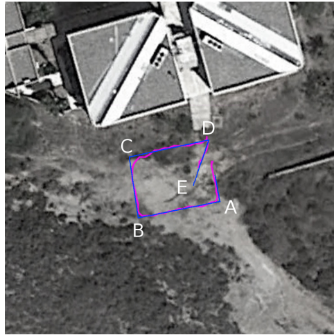
Fig. 6. The paths followed by the target color object and the robot, at the Object Following testing scenario, are marked blue and pink respectively. The errors are due to the hysteresis of the robot's locomotion system.
