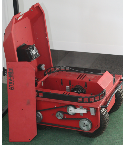
Fig. 3. The reconstruction procedure left robot's frame, wheels, electrical motors, and transmission unchanged.
