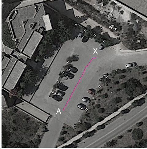
Fig. 4. The experimental testing scenario for the Move To Point node was driving the robot from its current position X, straight to POI A, travelling a distance of 30m using half speed - approximately 5.2km/h. The path followed by the robot is shown in magenta. The mean error value, i.e. the distance from the straight path, was 0.8m and it is due to errors at the GPS readings.
