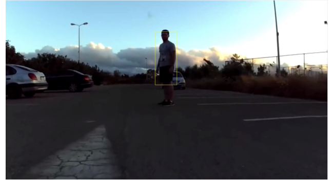
Fig. 6. Pedestrian detection using stereo camera
