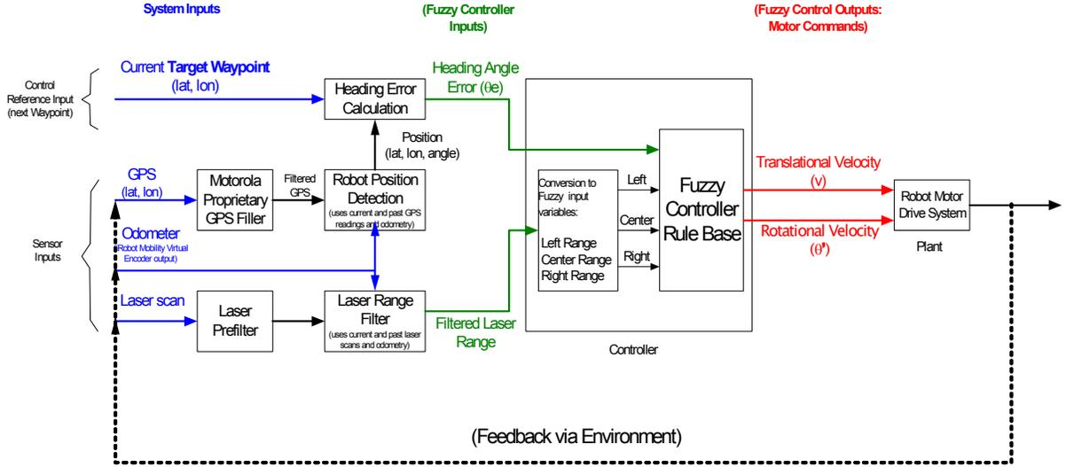
Fig. 3. Controller Block Diagram
