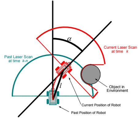
Fig. 2: Laser scans taken at time  $k$  (most recent scan) and at time  $k-n$  (a previous scan).
