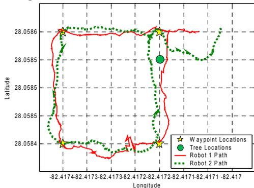
Fig. 6: Path followed by the two robots in the second experiment
