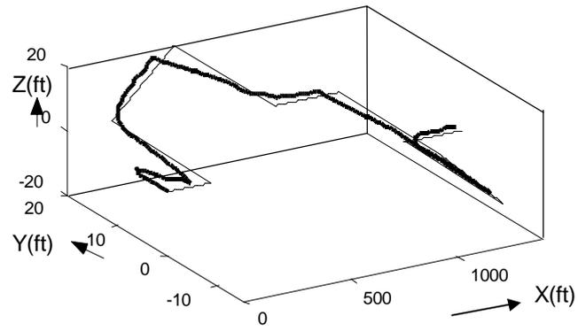
Figure 6: Test case 2: Ordered and actual path with lateral current velocity 0.8 ft/sec
