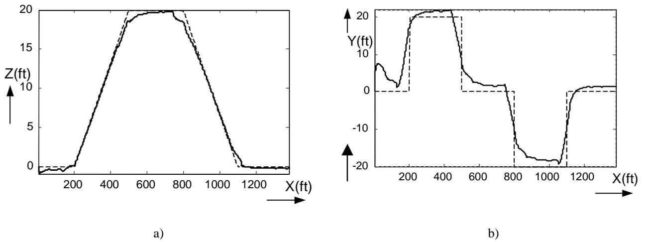
Figure 7: Test case 2: Ordered and actual path in (a) XZ plane and (b) XY plane with lateral current velocity 0.8 ft/sec
