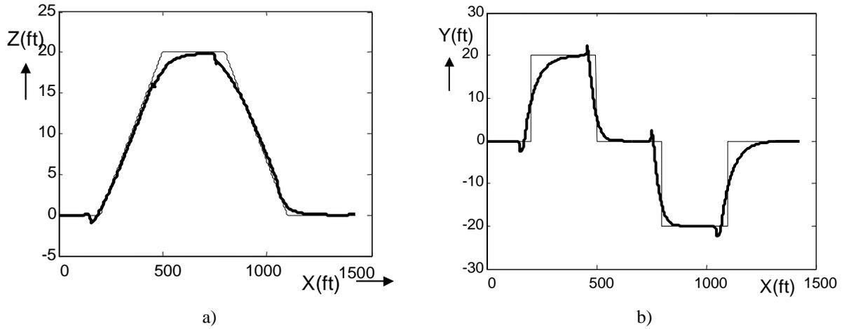
Figure 3: Test case 1: Ordered and actual path in (a) the vertical and (b) the horizontal plane
