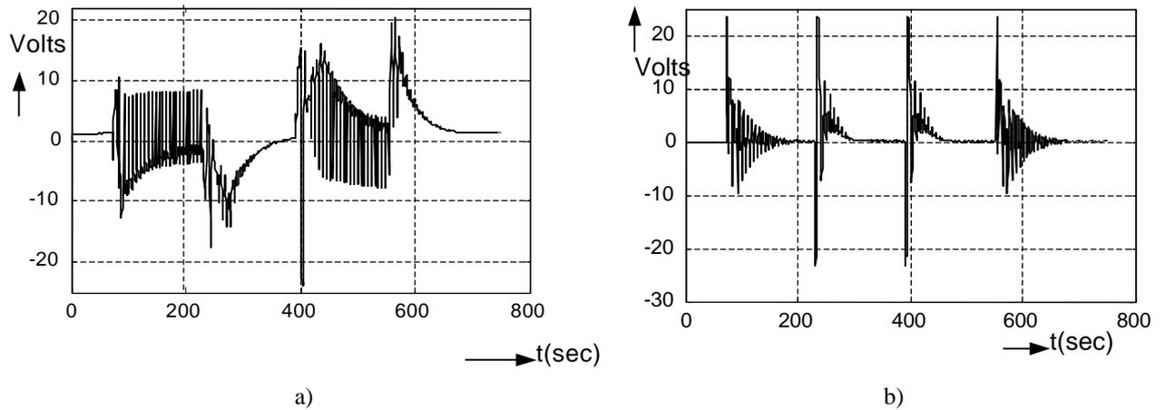
Figure 4: Test case 1: (a) Vertical Bow Thruster Voltage and (b) Lateral Bow Thruster Voltage versus time
